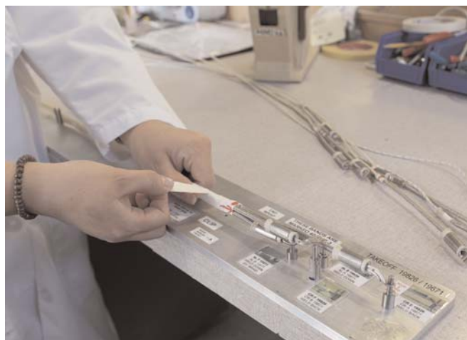
HIGH TEMPERATURE CABLE REPAIR.
